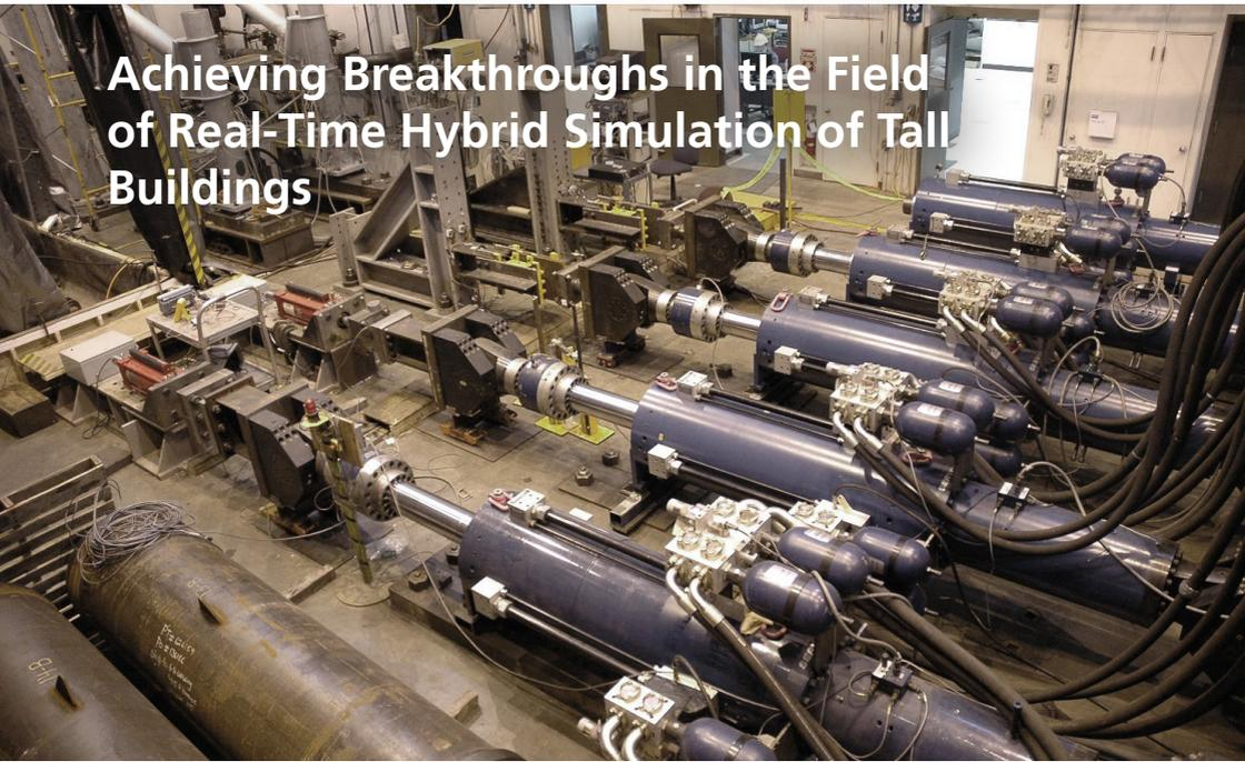
**In collaboration with Servotest, Natural Hazards Engineering Research Infrastructure (NHRI) Experimental Facility (EF) at Lehigh University has developed a MATLAB® and Simulink® based algorithm and deployed it to Speedgoat hardware to perform real-time hybrid simulations of tall buildings excited by wind or seismic forces.**
